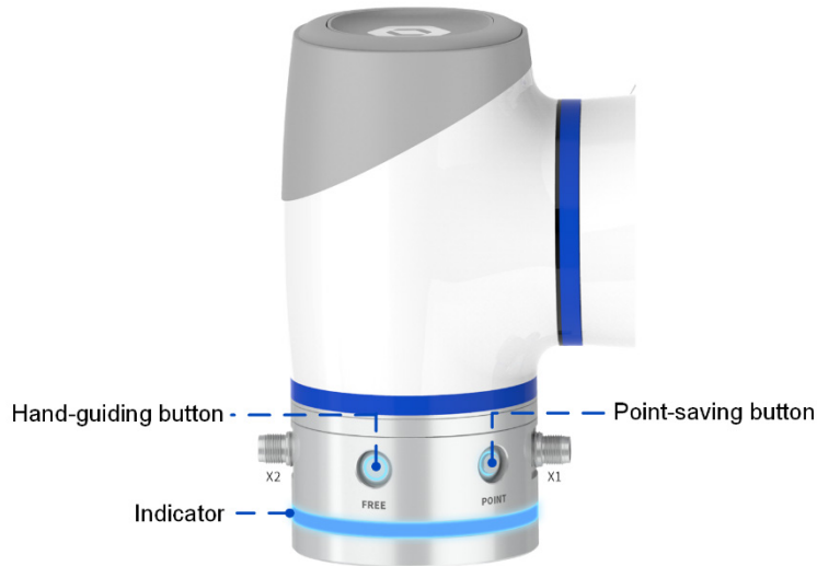
Figure 2.8 Tool flange buttons and indicator (CR20A/CR20AF/CR30A)
