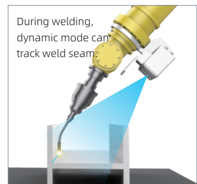
Dynamic Mode: The object being measured moves relative to the camera, and the laser line sweeps over the object to complete the scan.
