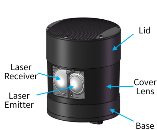
Figure 1. Partial cross-sectional diagram
