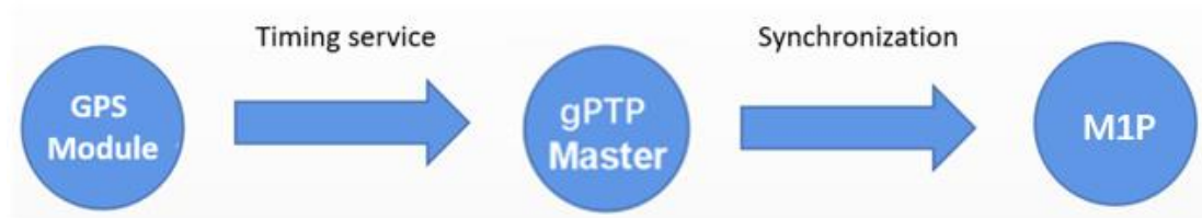
Figure 6: Topology of GPS Timing service synchronization
