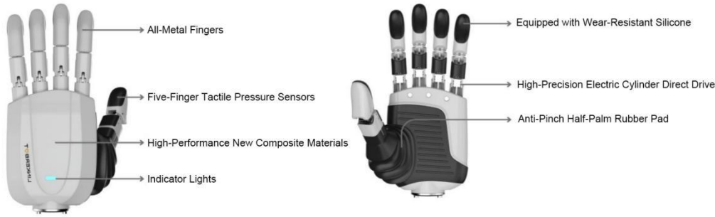
Figure 1-2. Structure and Characteristics Display Diagram of Linker Hand L6
