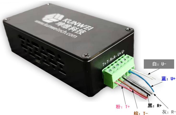
Fig.6 Diagram of the serial server wiring
